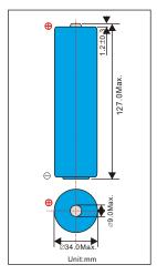
NOTE! ER341245S is High temperature Type batterywhich has extended temperature range up to 150°C. It may require depassivation before high currents can be delivered.
